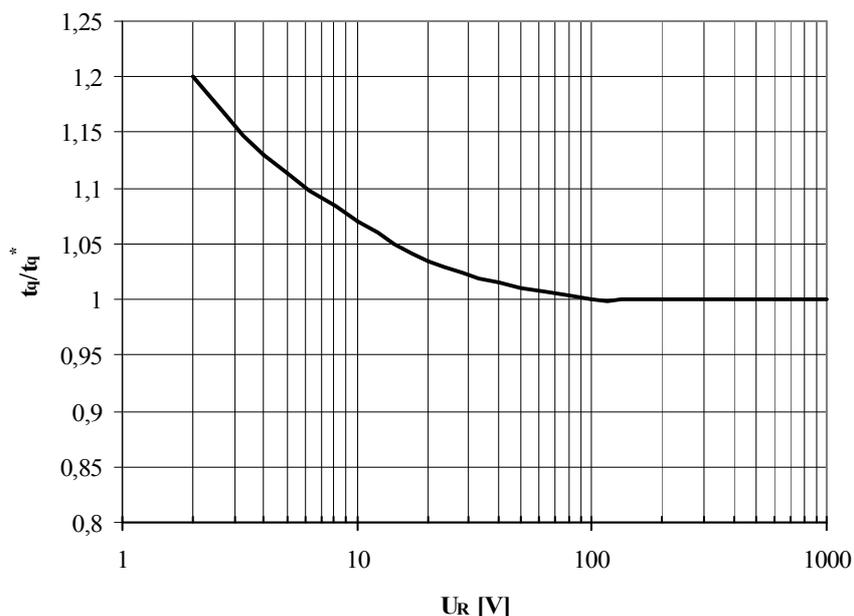
**Fig. 5** Turn-off time  $t_q$  vs. Reverse voltage  $V_R$
