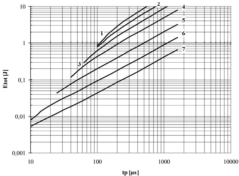
**Fig. 24** Square wave loss energy per pulse
