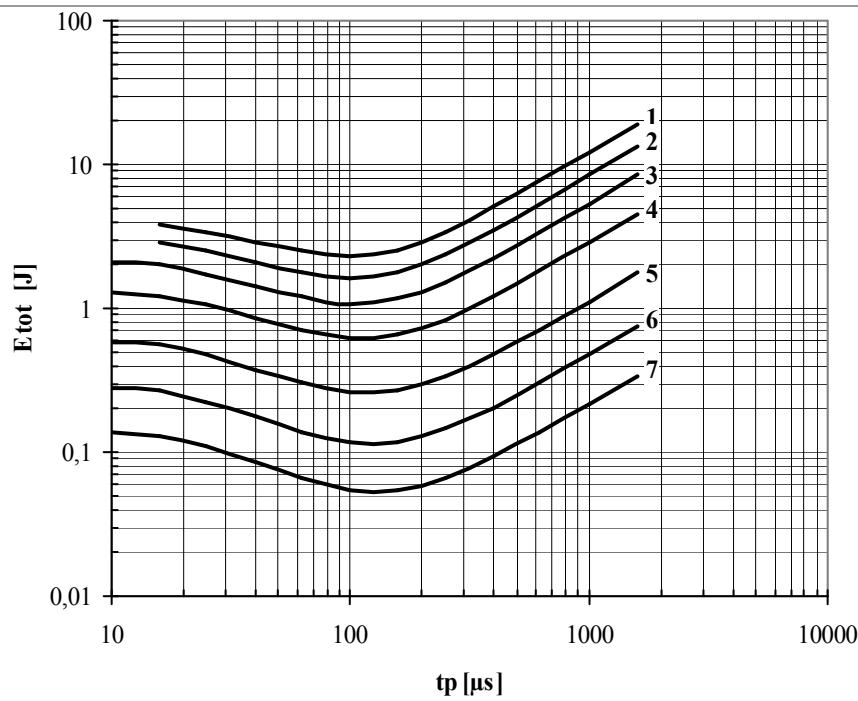
**Fig. 23** Sine wave loss energy per pulse
