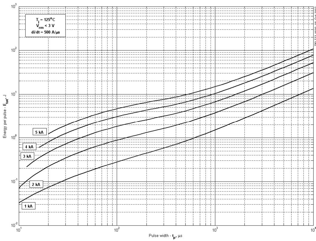
Fig 21 – Square wave energy per pulse
