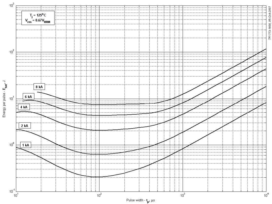
Fig 11 – Sine wave energy per pulse
