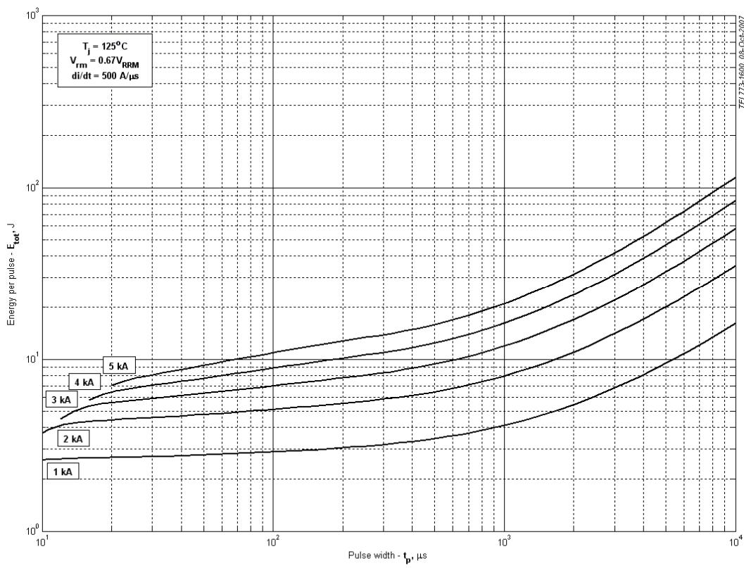
Fig 27 – Square wave energy per pulse
