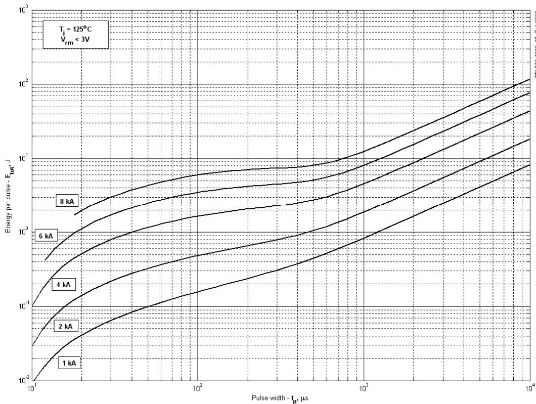
Fig 10 – Sine wave energy per pulse
