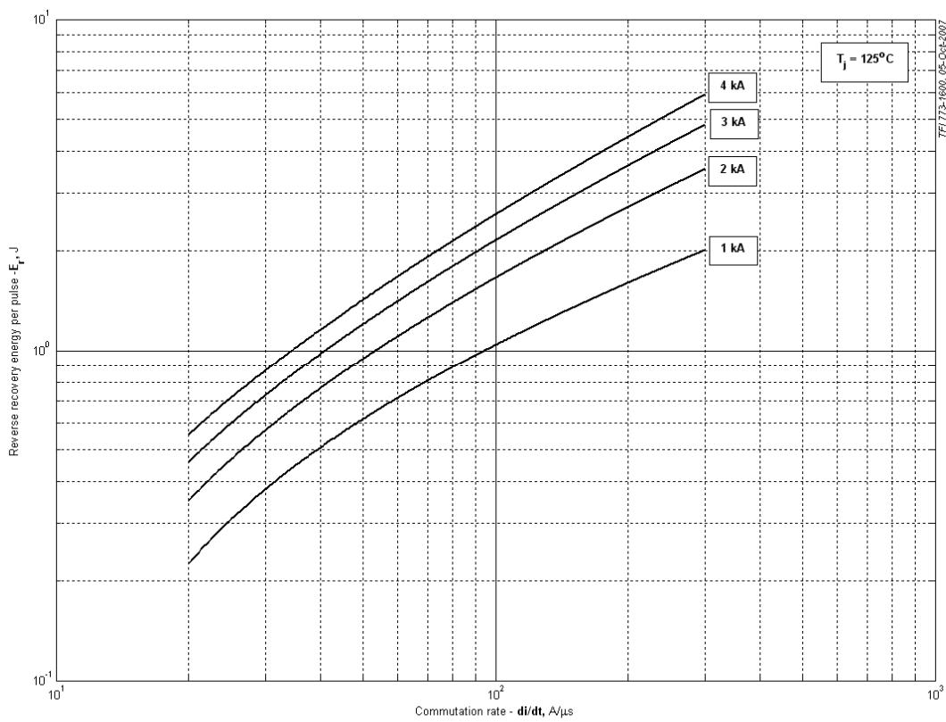
Fig 9 – Reverse recovery energy per pulse
