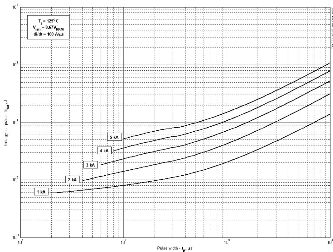
Fig 26 – Square wave energy per pulse
