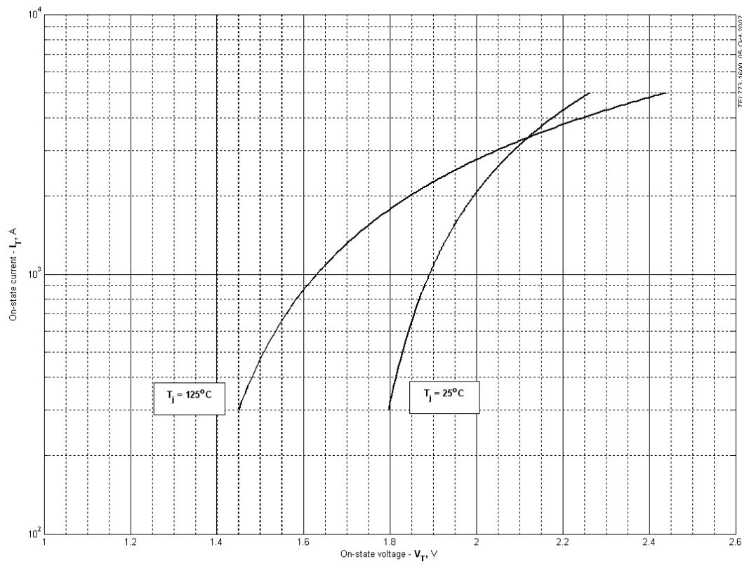
Fig 1 – On-state characteristics of Limit device
