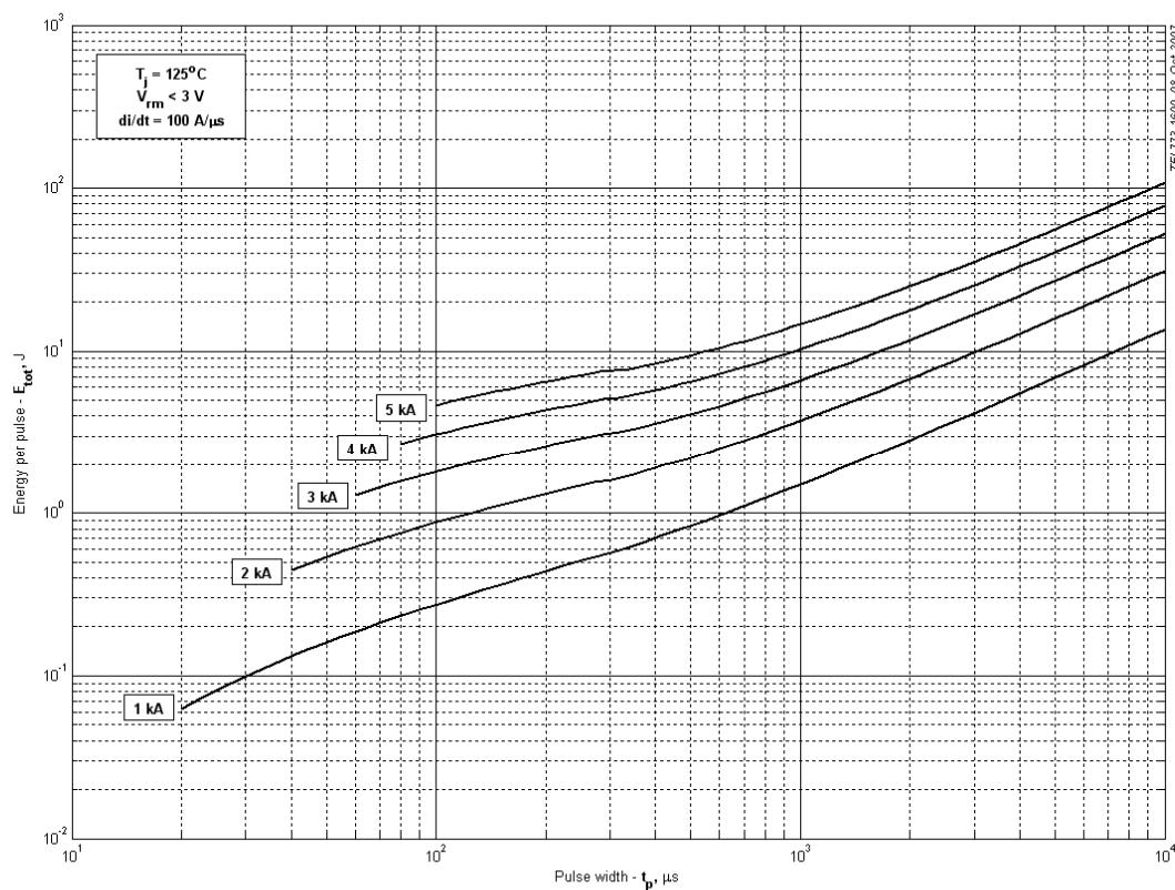
Fig 20 – Square wave energy per pulse
