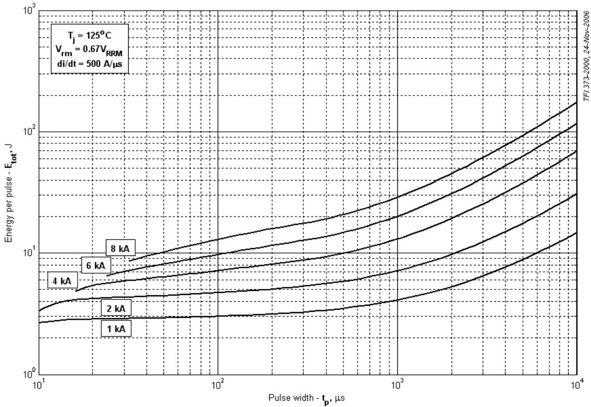
Fig 27 – Square wave energy per pulse
