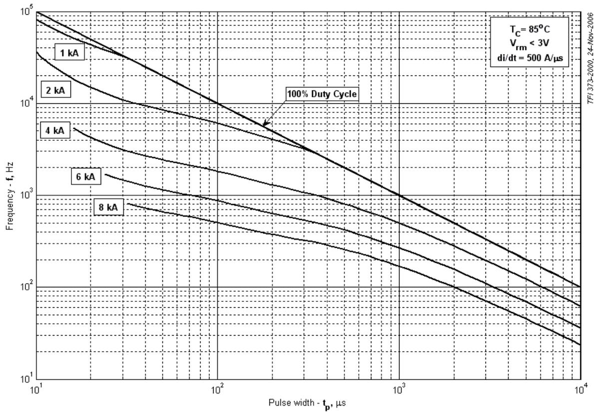
Fig 19 – Square wave frequency ratings
