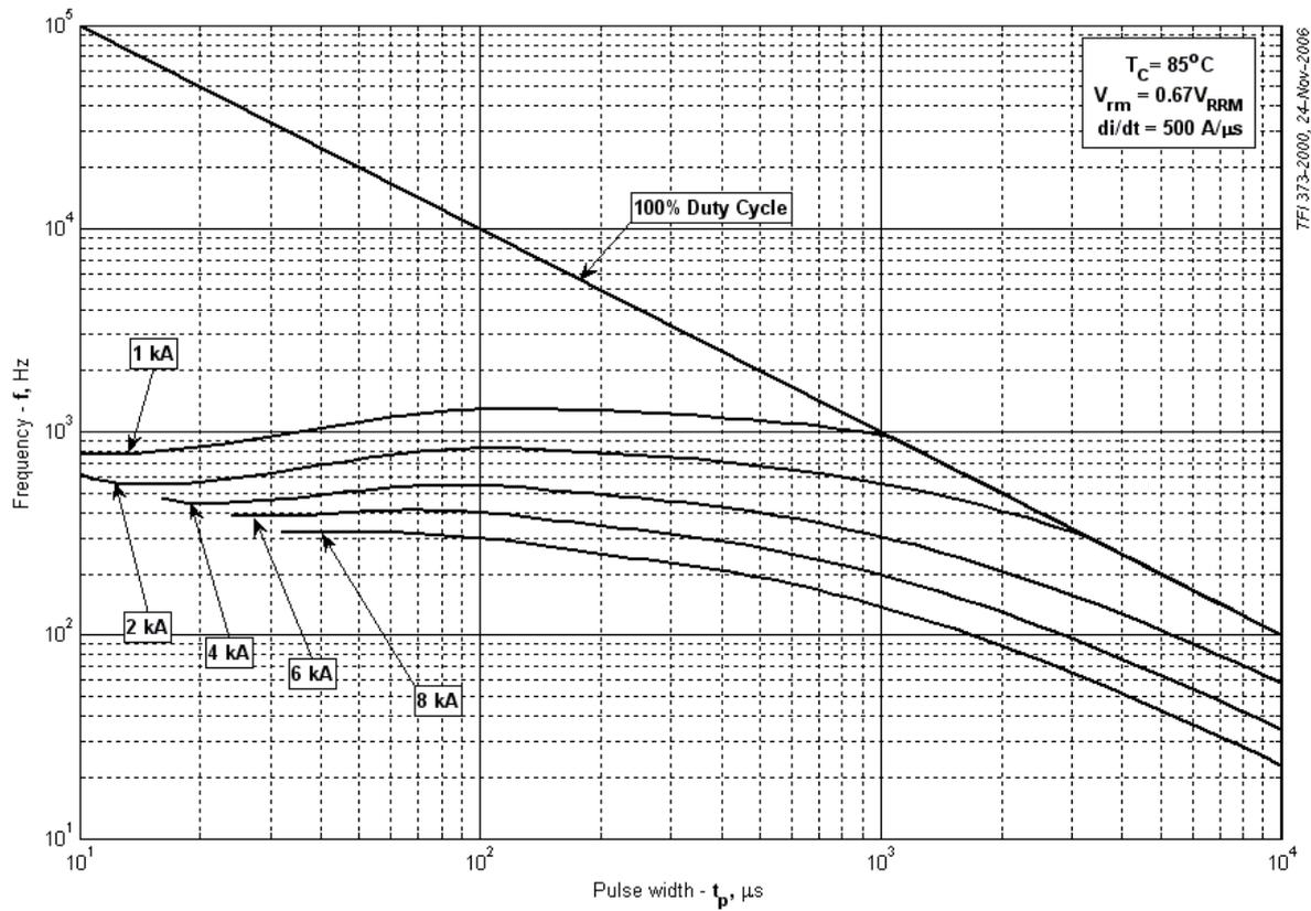
Fig 25 – Square wave frequency ratings
