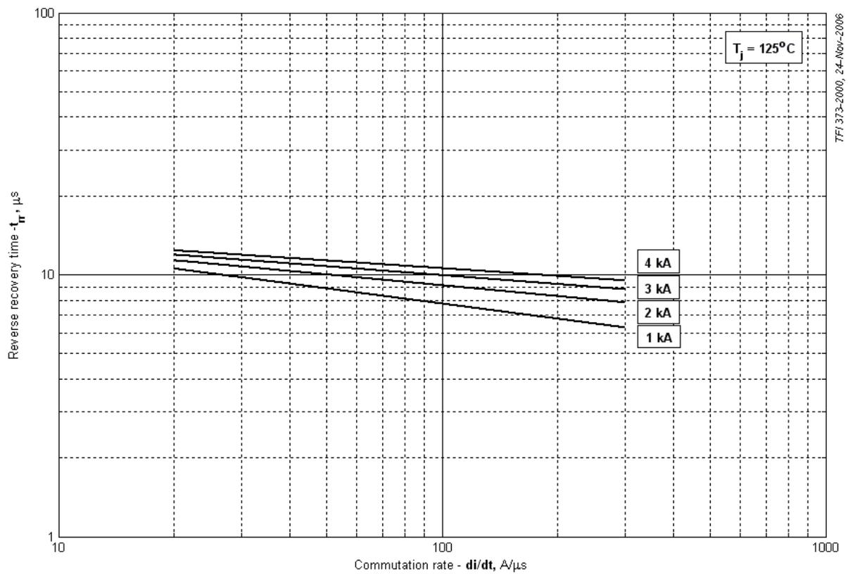
Fig 8 – Maximum recovery time,  $t_{tr}$  (linear)
