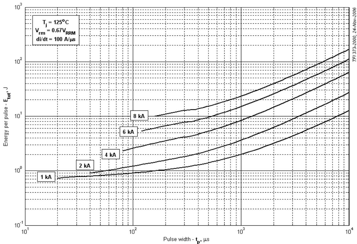
Fig 26 – Square wave energy per pulse
