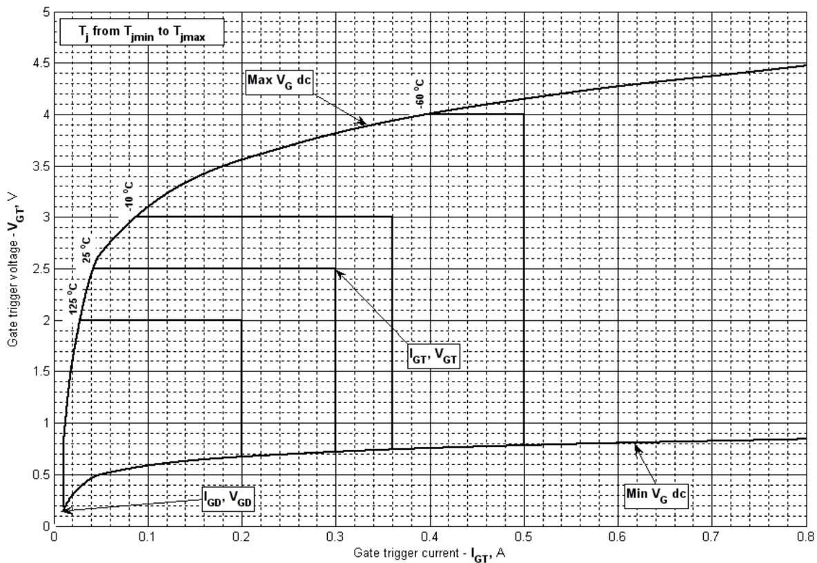
Fig 3 – Gate characteristics – Trigger limits
