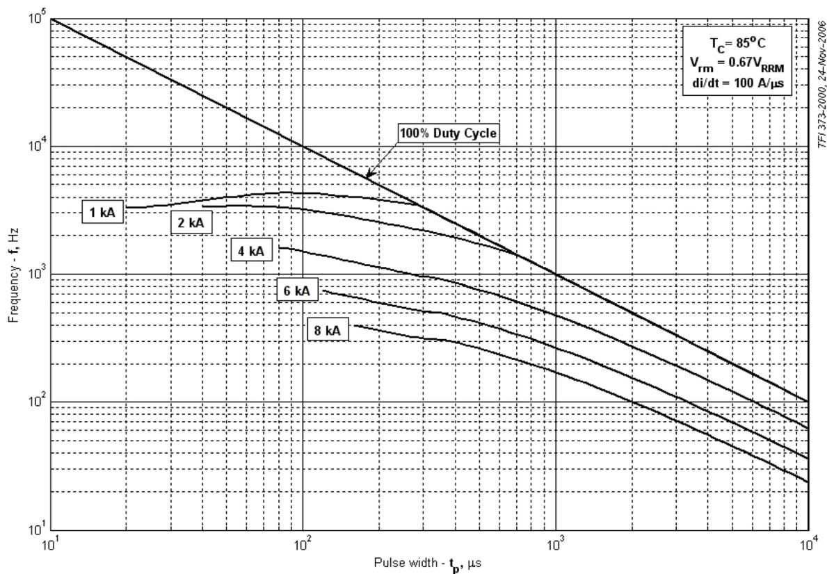
Fig 24 – Square wave frequency ratings
