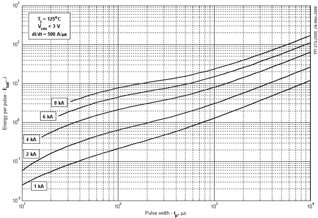
Fig 21 – Square wave energy per pulse
