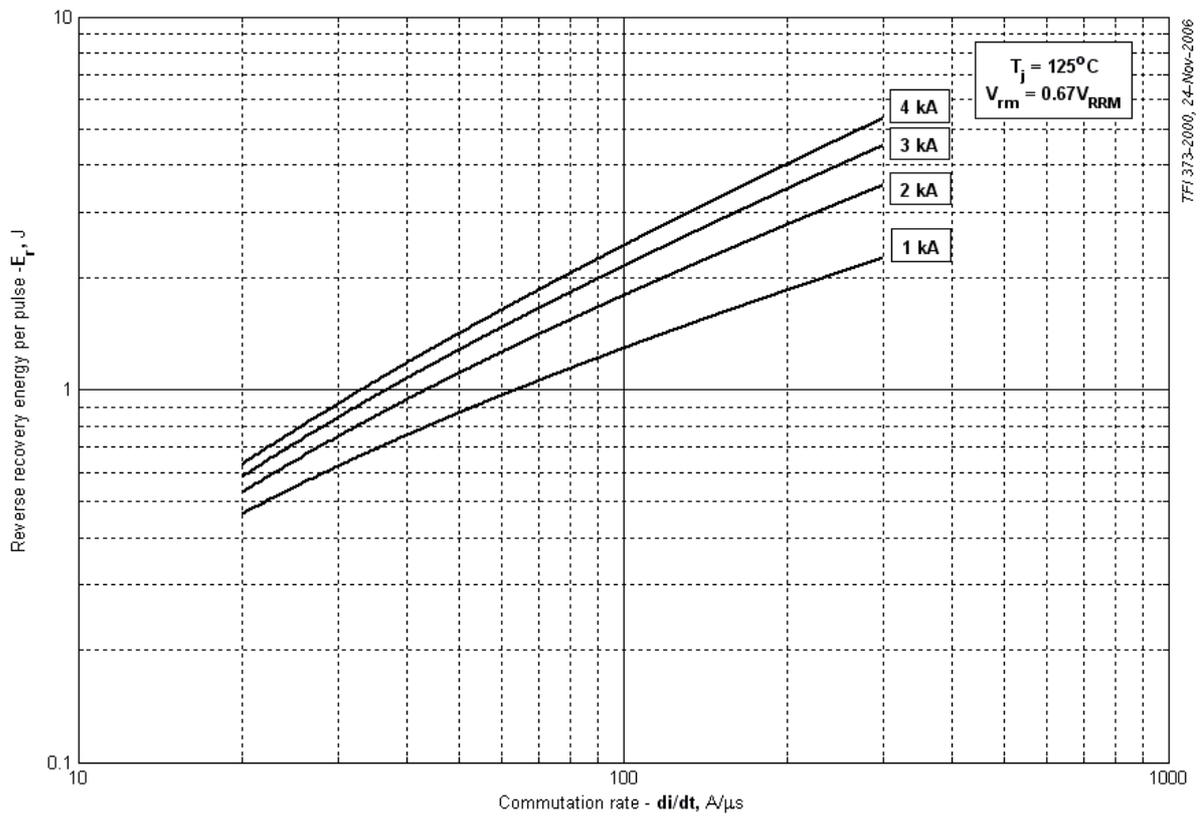
Fig 9 – Reverse recovery energy per pulse
