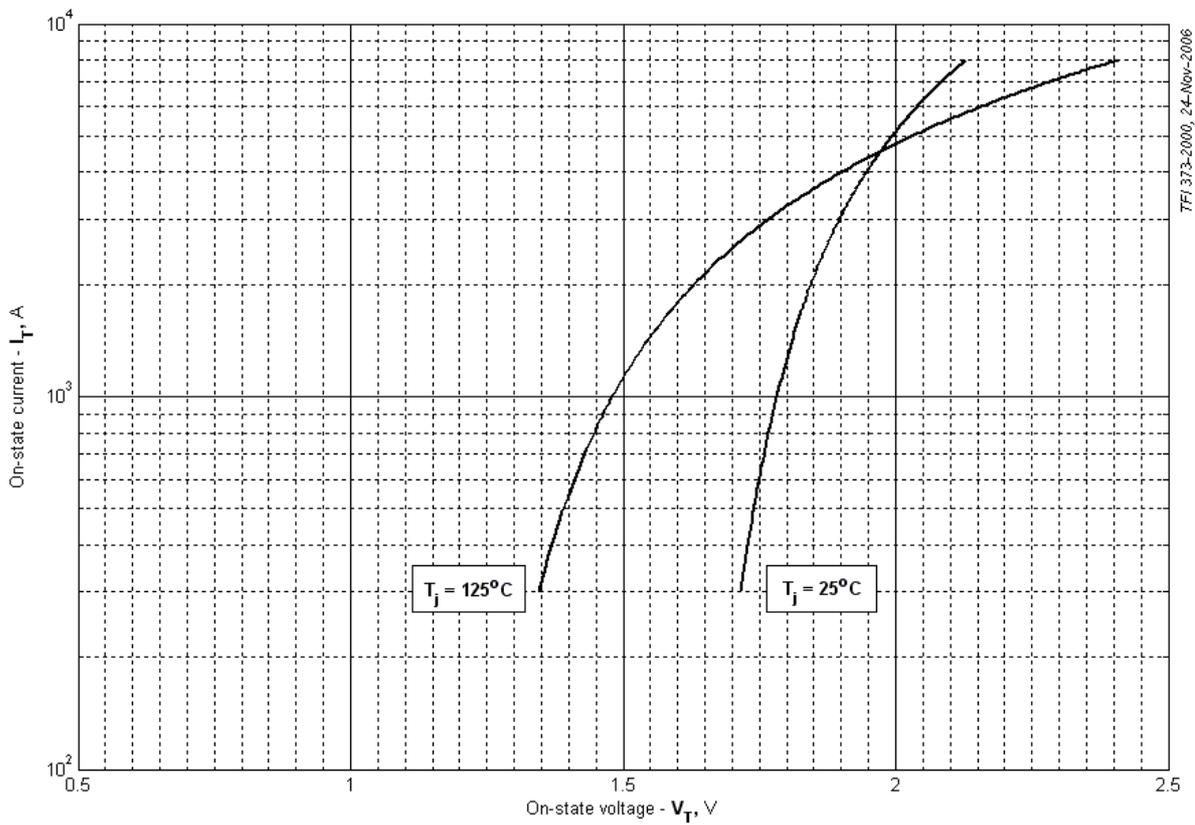
Fig 1 – On-state characteristics of Limit device
