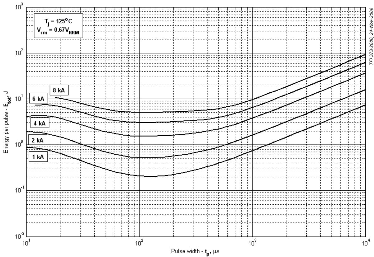
Fig 11 – Sine wave energy per pulse
