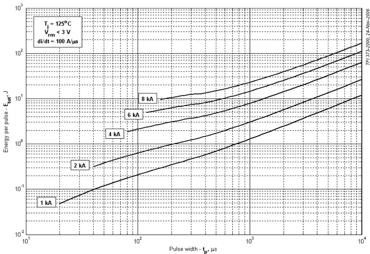
Fig 20 – Square wave energy per pulse
