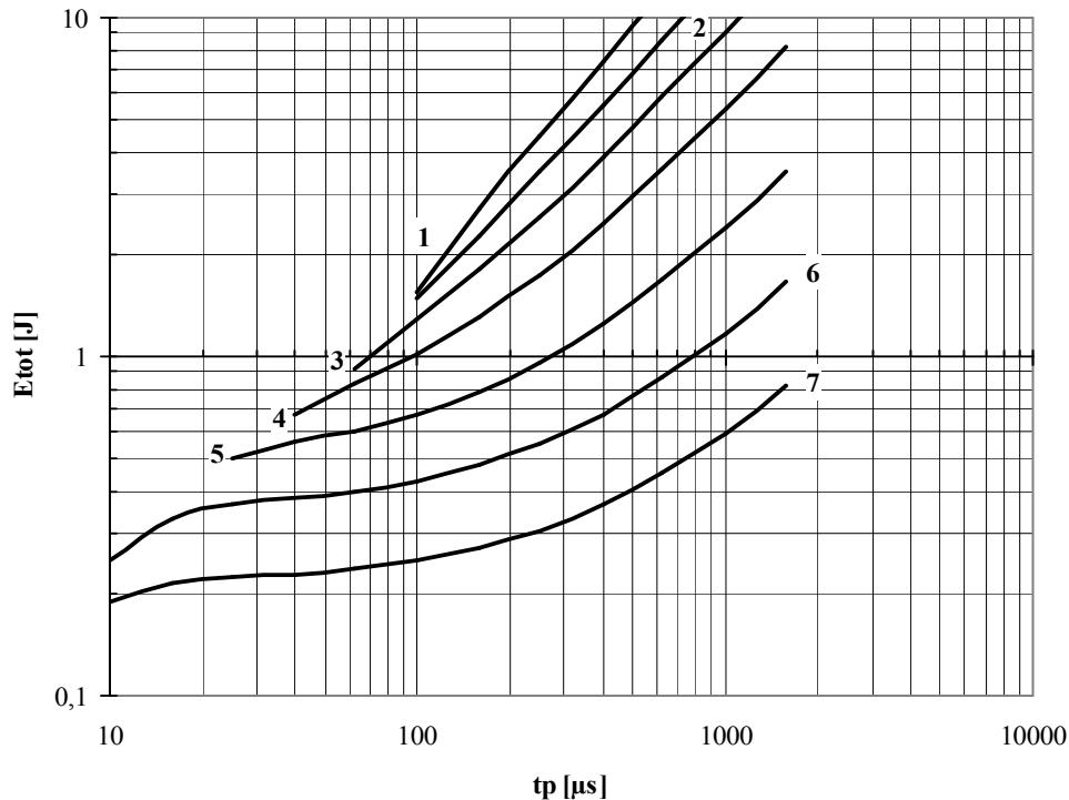
**Fig. 26** Square wave loss energy per pulse
