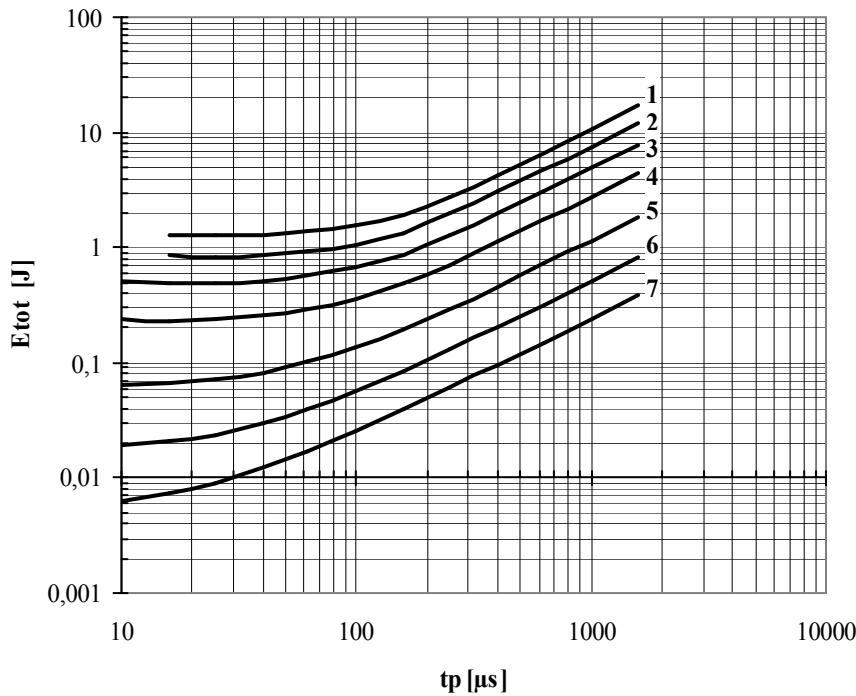
**Fig. 22** Sine wave loss energy per pulse
