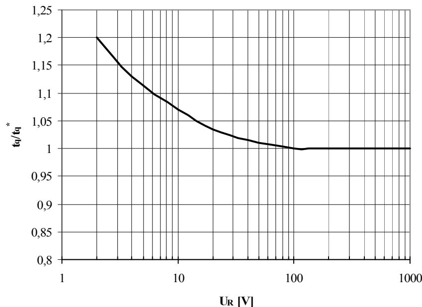
**Fig. 5** Turn-off time  $t_q$  vs. Reverse voltage  $V_R$
