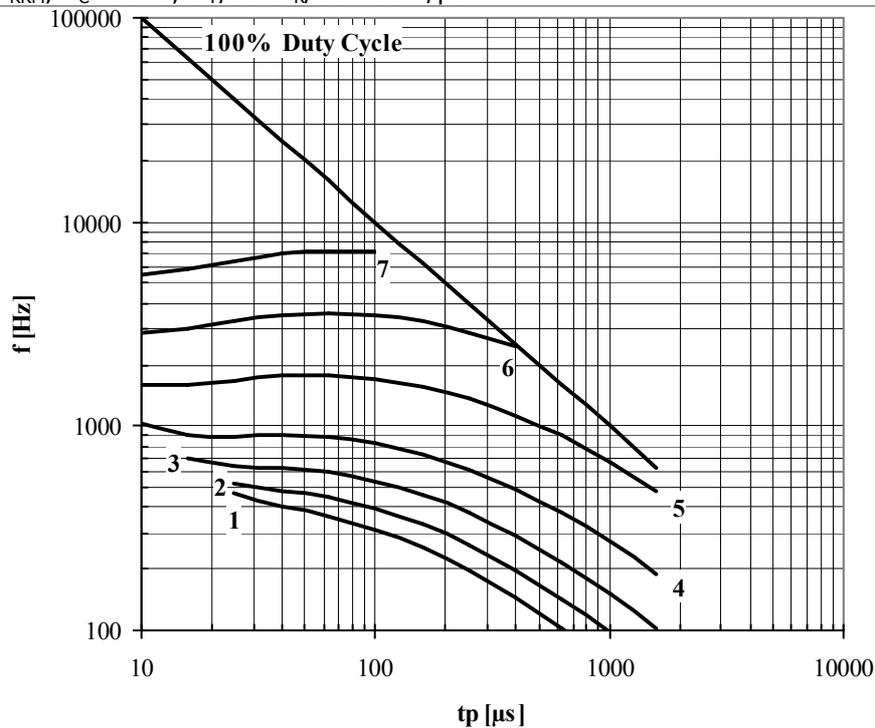
**Fig. 19** Square wave frequency ratings
