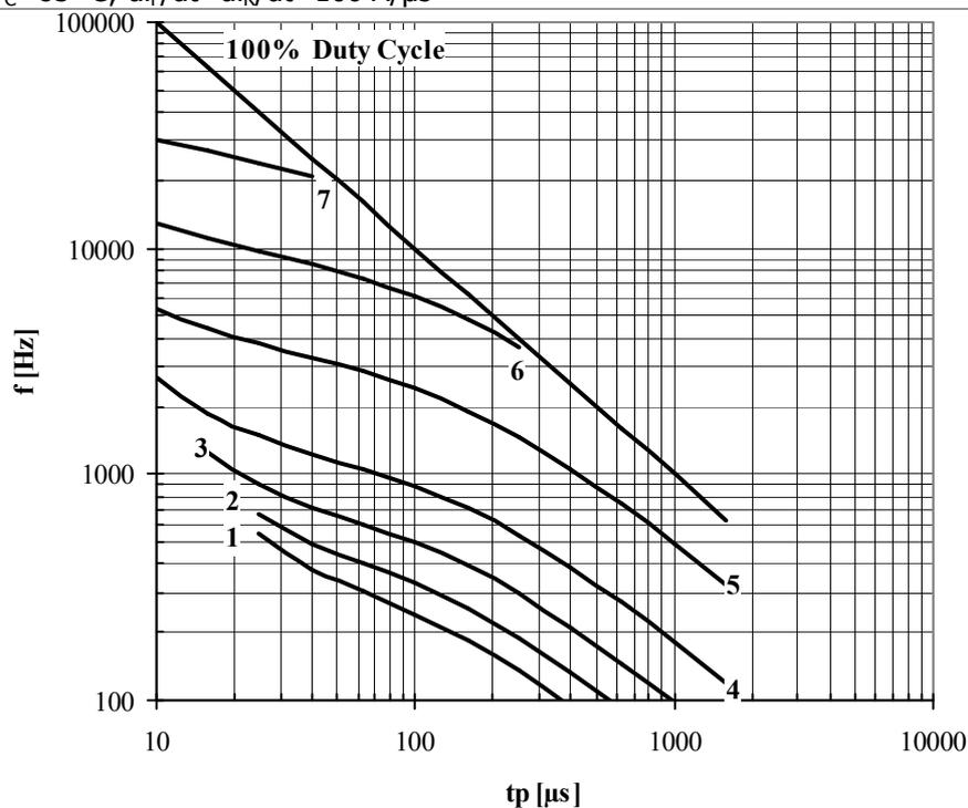
**Fig. 17** Square wave frequency ratings
