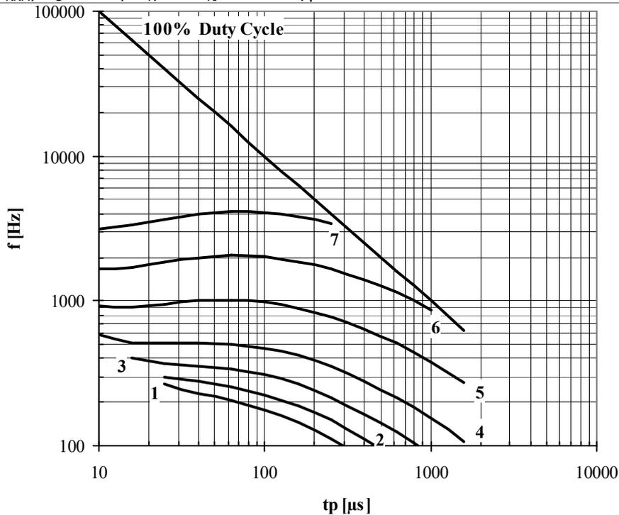
**Fig. 21** Square wave frequency ratings
