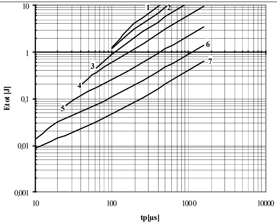
**Fig. 24** Square wave loss energy per pulse
