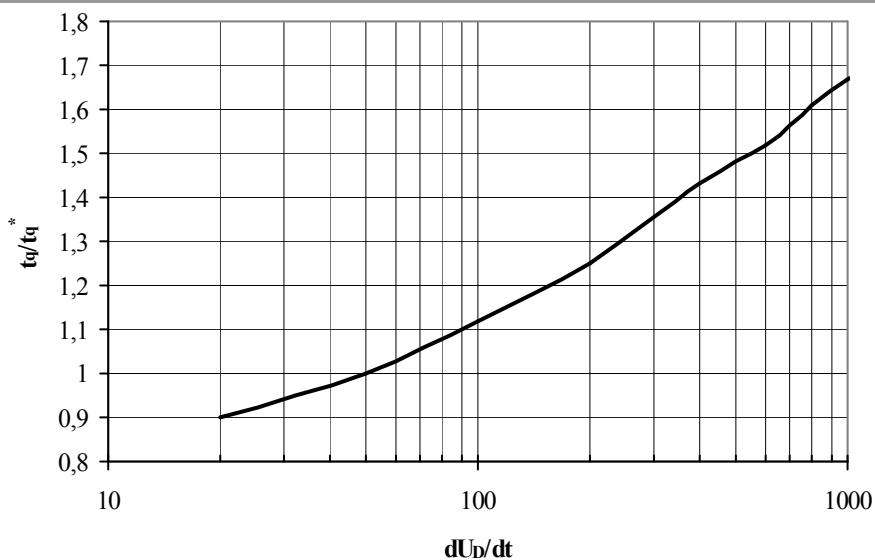
**Fig. 6** Turn-off time  $t_q$  vs. Rate of rise of commuting voltage  $dv_D/dt$
