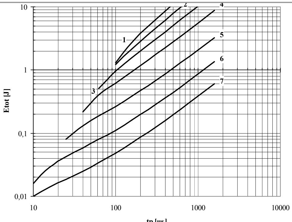
**Fig. 24** Square wave loss energy per pulse
