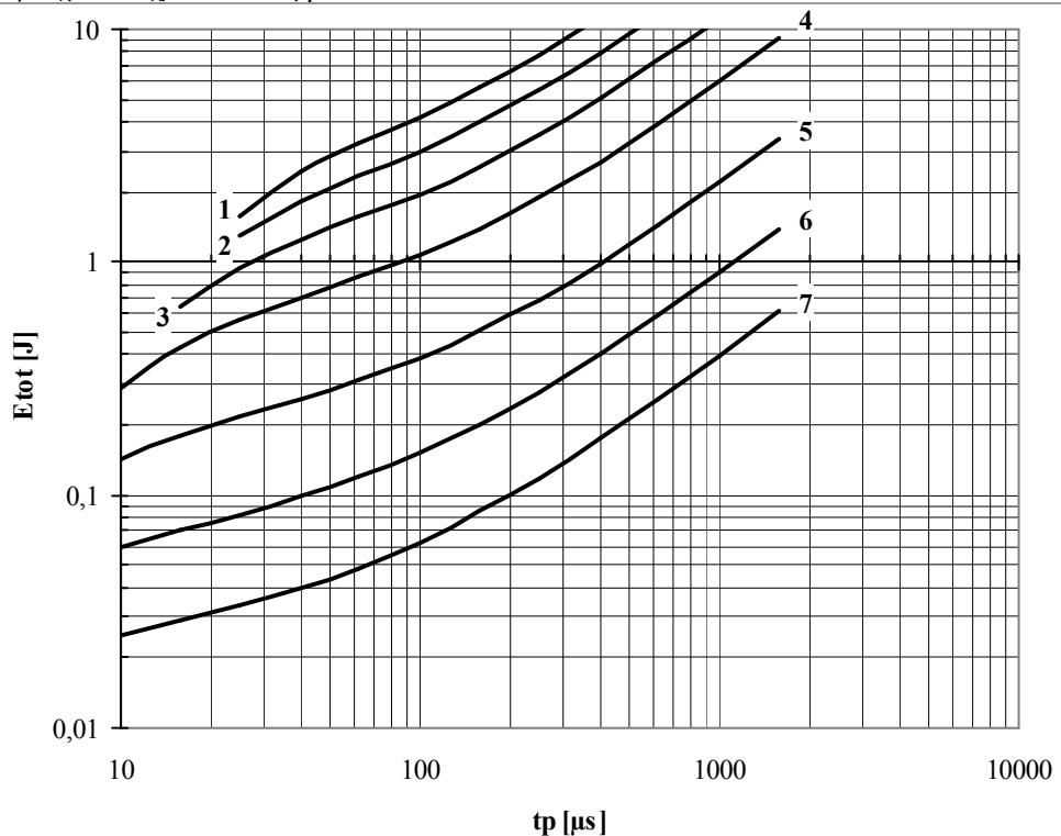
**Fig. 25** Square wave loss energy per pulse
