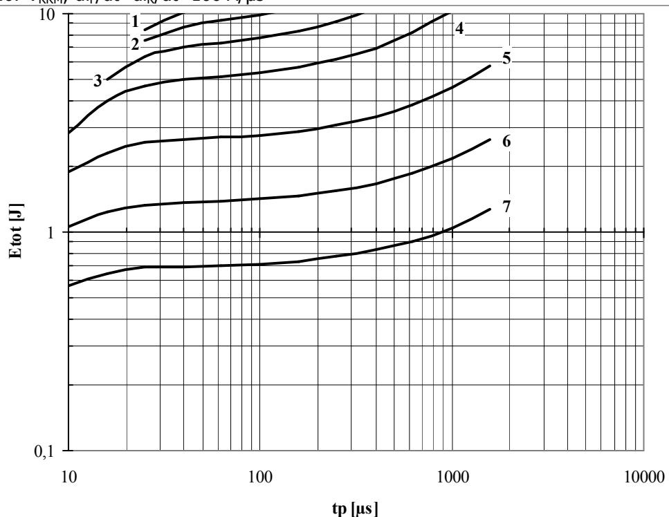
**Fig. 27** Square wave loss energy per pulse
