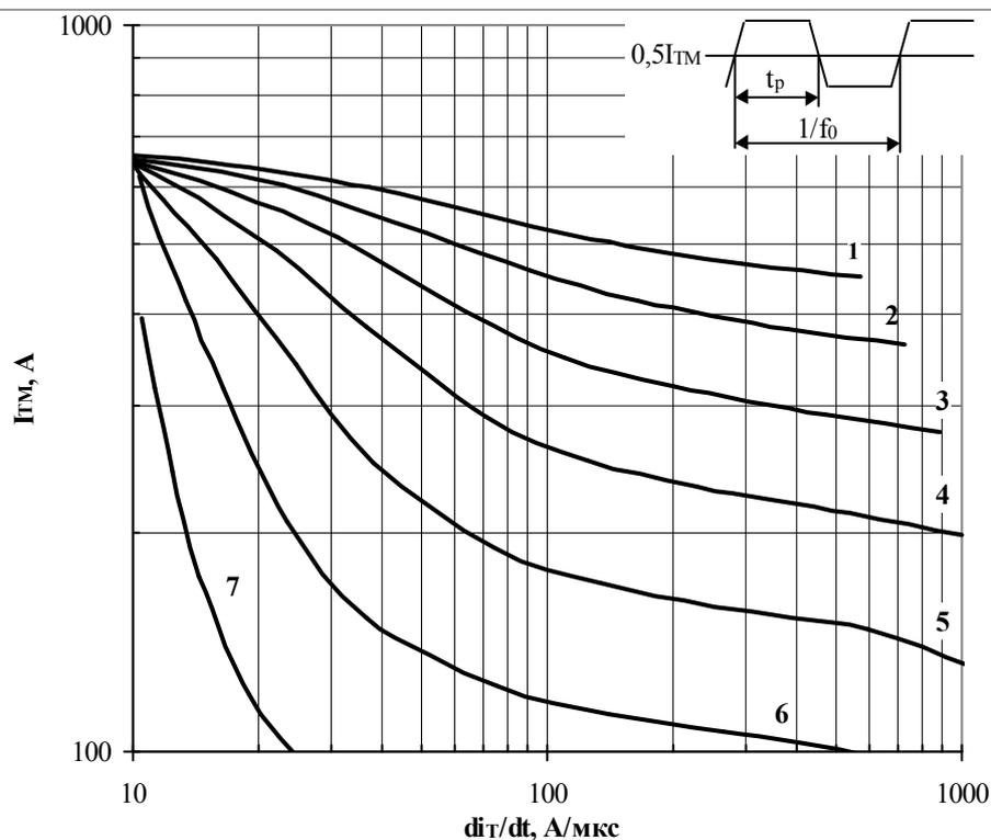
**Fig. 11** Maximum allowable mean on-state current  $I_{TM}$  of trapeze current waveform vs. on-state current rise rate  $di_T/dt$  for pulse duration  $t_p=1/2f_0$  and case temperature  $T_c=85\text{ }^\circ\text{C}$  at high frequency.
