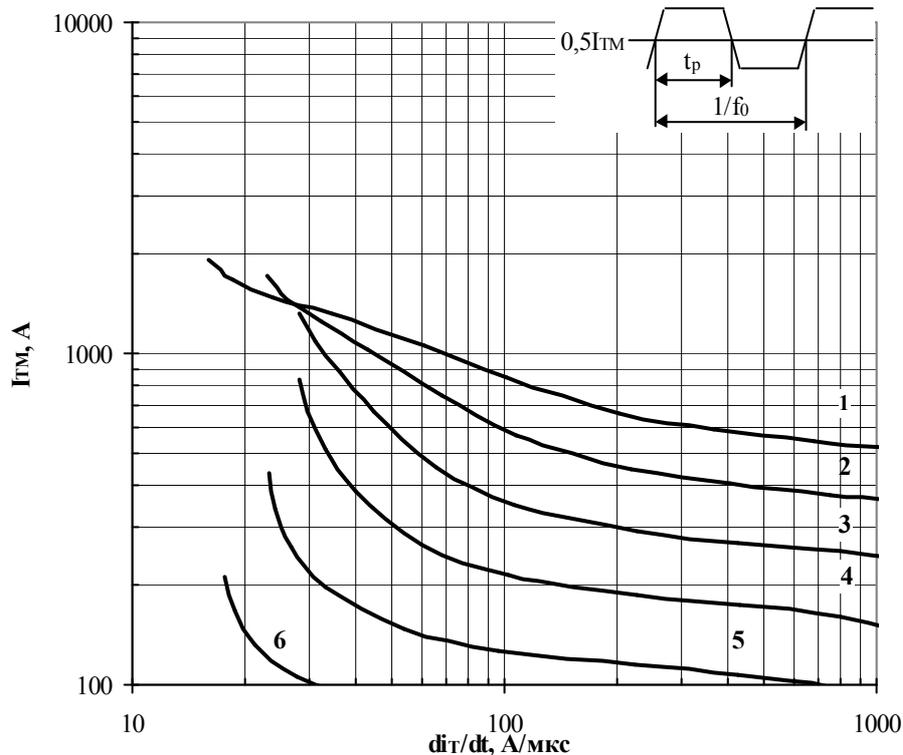
**Fig. 20** Maximum allowable mean on-state current  $I_{TAV}$  of trapeze current waveform vs. on-state current rise rate  $di_T/dt$  for pulse duration  $t_p=1/10f_0$ , cooling temperature  $T_a=40\text{ }^\circ\text{C}$ , cooling air force 6 m/s, heatsink 0143 at high frequency.
