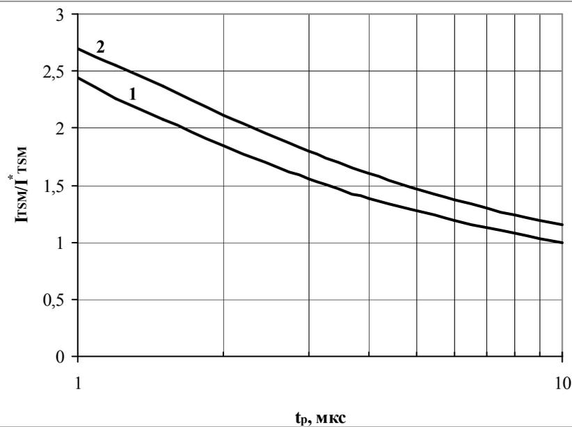
**Fig. 21** Maximum allowable surge on-state current  $I_{TM}$  vs. pulse duration  $t_p$ .
