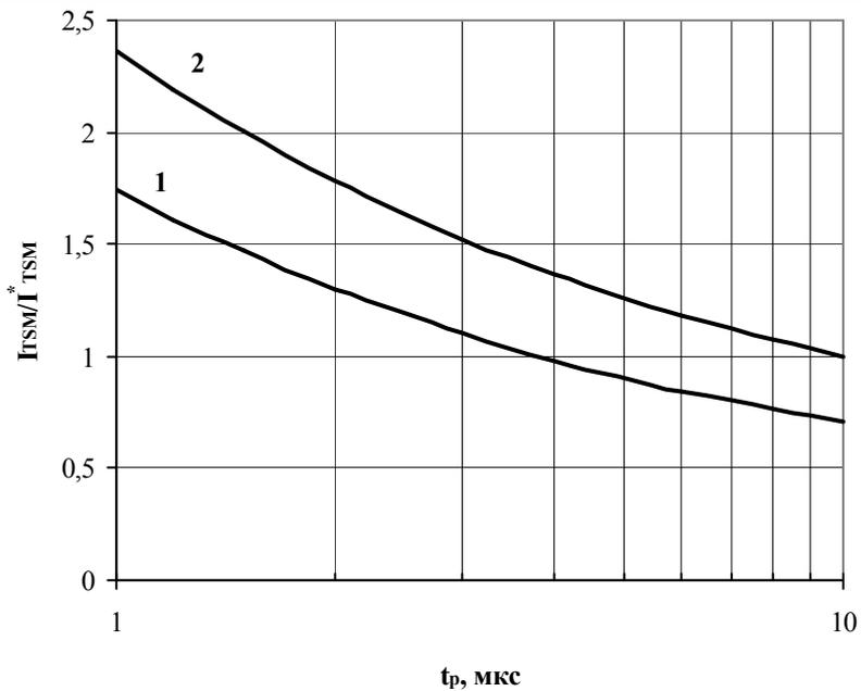
**Fig. 22** Maximum allowable surge on-state current  $I_{TM}$  vs. pulse duration  $t_p$  for initial junction temperature:
