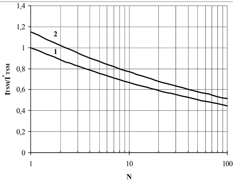
**Fig. 23** Maximum allowable surge on-state current  $I_{TM}$  vs. pulse quantity of overload current  $N$
