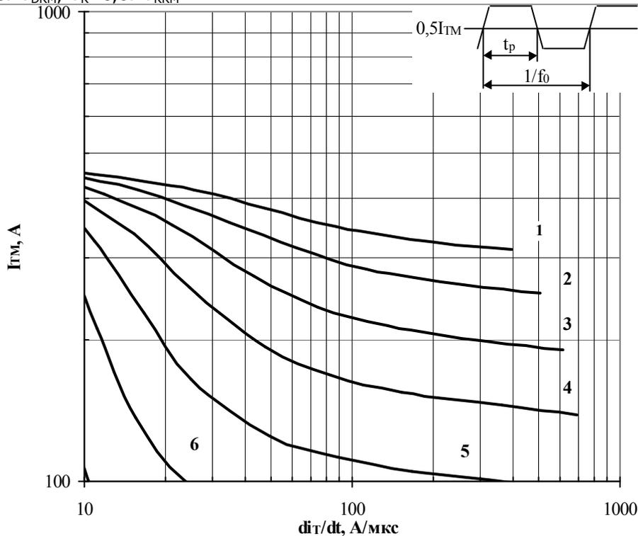
**Fig.18** Maximum allowable mean on-state current  $I_{TAV}$  of trapeze current waveform vs. on-state current rise rate  $di_T/dt$  for pulse duration  $t_p=1/2f_0$ , cooling temperature  $T_a=40\text{ }^\circ\text{C}$ , cooling air force 6 m/s, heat sink 0143 at high frequency.
