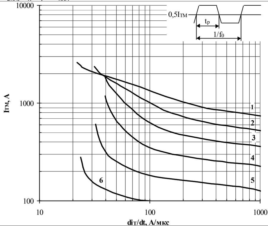
**Fig. 16** Maximum allowable mean on-state current  $I_{TM}$  of trapeze current waveform vs. on-state current rise rate  $di_T/dt$  for pulse duration  $t_p=1/10f_0$  and case temperature  $T_c=85$  °C at high frequency.
