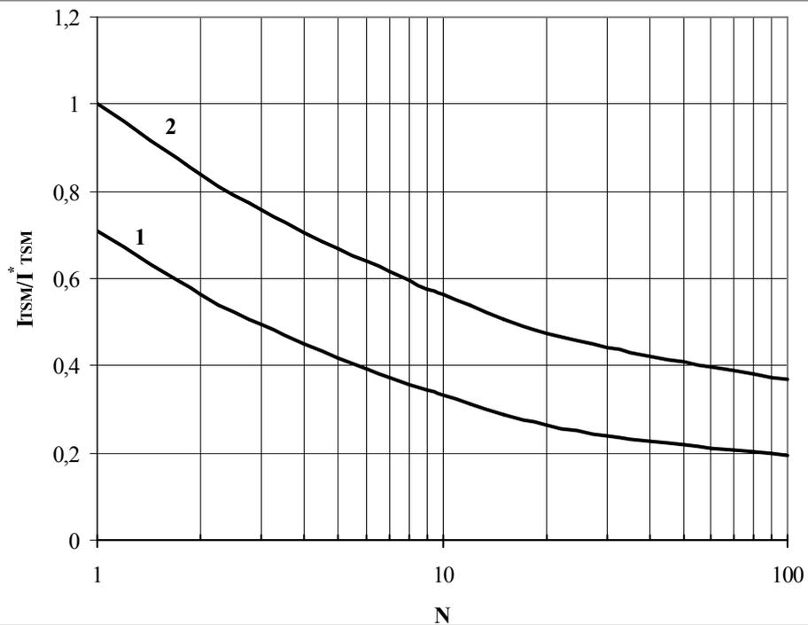
**Fig. 24** Maximum allowable surge on-state current  $I_{TM}$  vs. pulse quantity of overload current  $N$ .
