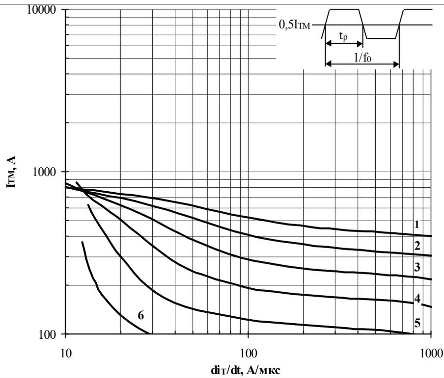
**Fig. 19** Maximum allowable mean on-state current  $I_{TAV}$  of trapeze current waveform vs. on-state current rise rate  $di_T/dt$  for pulse duration  $t_p=1/4f_0$ , cooling temperature  $T_a=40\text{ }^\circ\text{C}$ , cooling air force 6 m/s, heatsink 0143 at high frequency.
