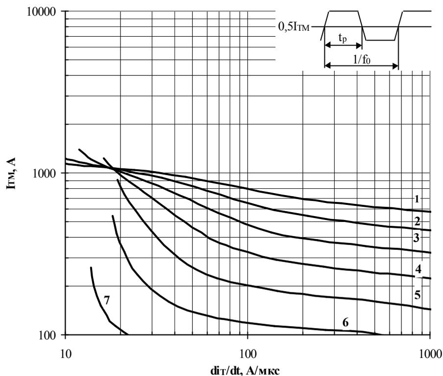
**Fig. 14** Maximum allowable mean on-state current  $I_{TM}$  of trapeze current waveform vs. on-state current rise rate  $di_T/dt$  for pulse duration  $t_p=1/4f_0$  and case temperature  $T_c=85\text{ }^\circ\text{C}$  at high frequency.
