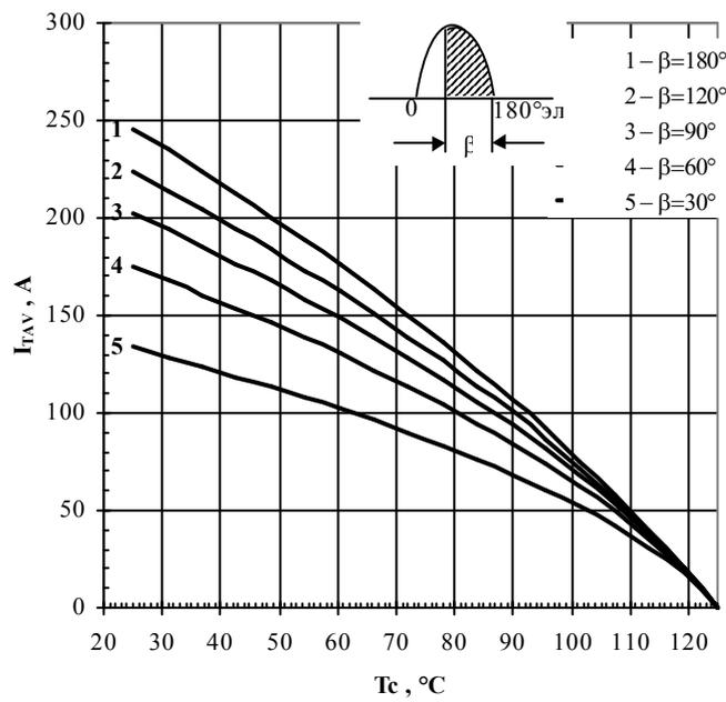
**Fig. 4** Maximum allowable mean on-state current  $I_{TAV}$  vs. cooling temperature  $T_a$  for cooling air force 6 m/s, heatsink O143 and sinusoidal current waveforms at different conduction angles,  $f=50\text{Hz}$
