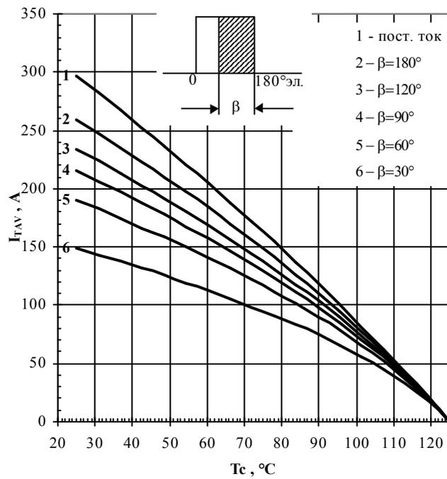
**Fig. 5** Maximum allowable mean on-state current  $I_{TAV}$  vs. cooling temperature  $T_a$  for cooling air force 6 m/s, heatsink O143 and rectangular current waveforms at different conduction angles,  $f=50\text{Hz}$
