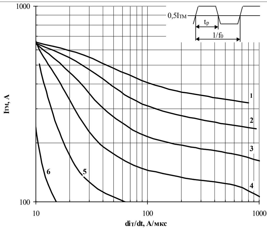
**Fig. 15** Maximum allowable mean on-state current  $I_{TM}$  of trapeze current waveform vs. on-state current rise rate  $di_T/dt$  for pulse duration  $t_p=1/4f_0$  and case temperature  $T_c=105$  °C at high frequency.
