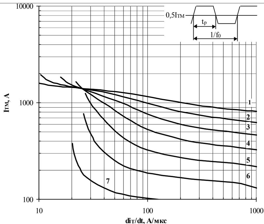
**Fig. 13** Maximum allowable mean on-state current  $I_{TM}$  of trapeze current waveform vs. on-state current rise rate  $di_T/dt$  for pulse duration  $t_p=1/4f_0$  and case temperature  $T_c=65\text{ }^\circ\text{C}$  at high frequency.
