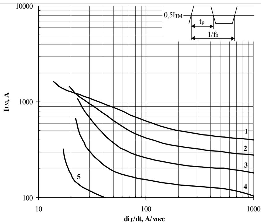
**Fig. 17** Maximum allowable mean on-state current  $I_{TM}$  of trapeze current waveform vs. on-state current rise rate  $di_T/dt$  for pulse duration  $t_p=1/10f_0$  and case temperature  $T_c=105\text{ }^\circ\text{C}$  at high frequency.
