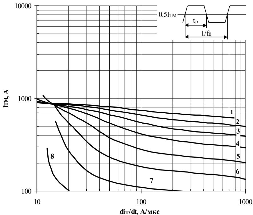
**Fig. 10** Maximum allowable mean on-state current  $I_{TM}$  of trapeze current waveform vs. mean on-state current  $di_T/dt$ , pulse duration  $t_p=1/2f_0$  and case temperature  $T_c=65\text{ }^\circ\text{C}$ .
