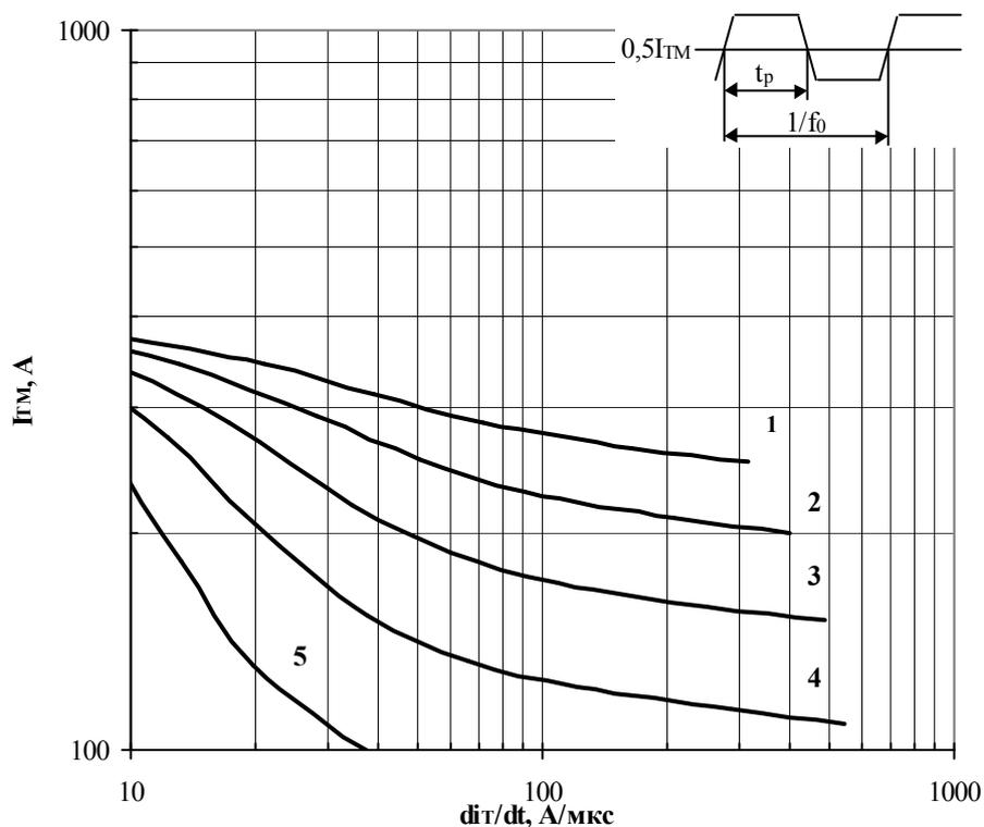
**Fig. 12** Maximum allowable mean on-state current  $I_{TM}$  of trapeze current waveform vs. on-state current rise rate  $di_T/dt$  for pulse duration  $t_p=1/2f_0$  and case temperature  $T_c=105\text{ }^\circ\text{C}$  at high frequency.
