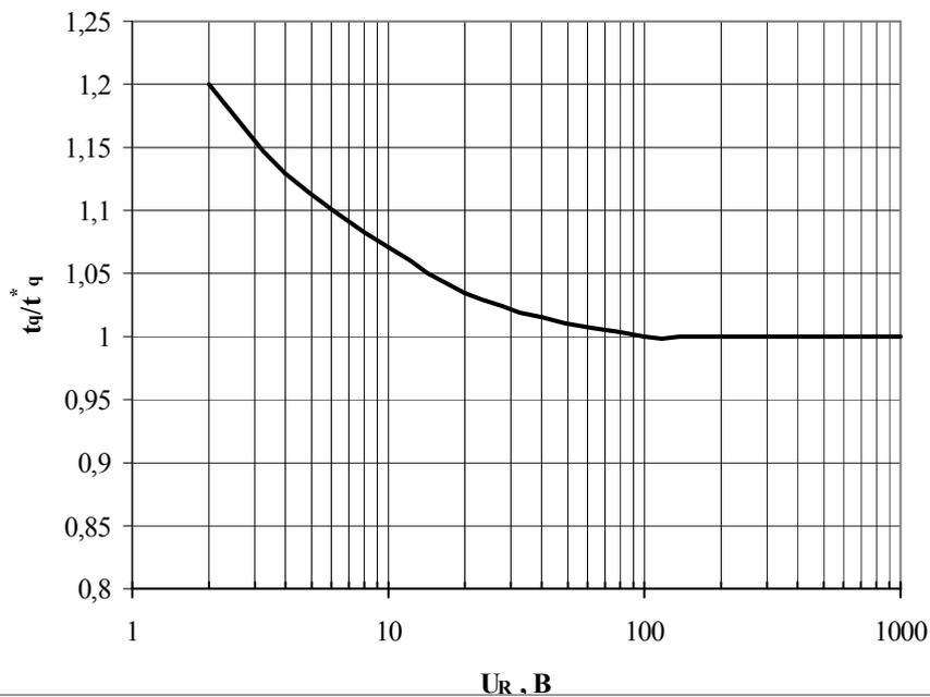
**Fig. 27** Turn-on time  $t_q$  vs. reverse voltage  $V_R$ .
