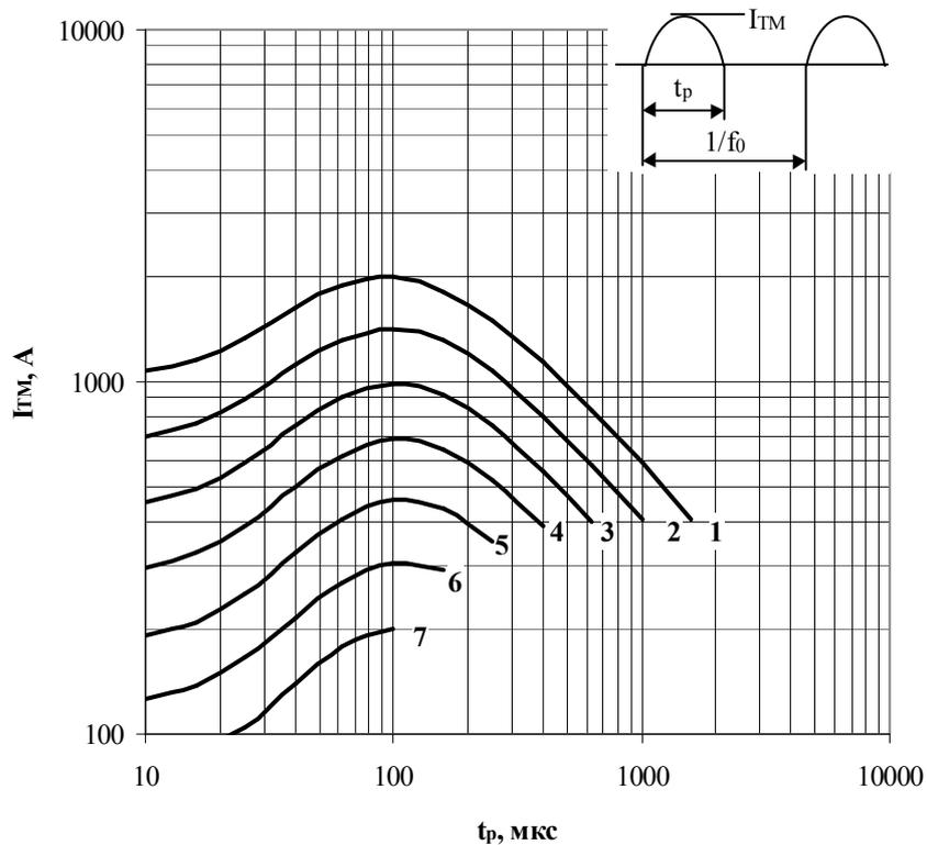
**Fig. 9** Maximum allowable mean on-state current  $I_{TAV}$  of sinusoidal current waveform vs. pulse duration  $t_p$  for cooling temperature  $T_a=40\text{ }^\circ\text{C}$ , cooling air force 6 m/s, heat sink 0143 at high frequency.
